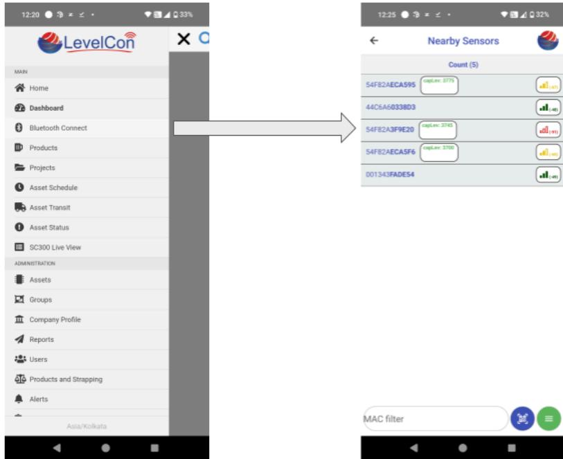
3. Select the appropriate device address that you wish to connect to from the nearby sensors list. On successful connection you'll be greeted with the status page of the. By default LevelCon devices come pre configured from the factory. We will now move to the log tab to view the device log messages
