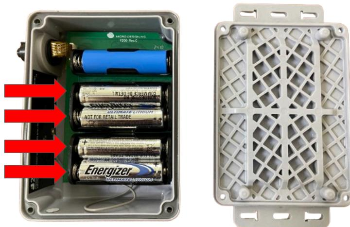
3. Once the batteries are replaced, make sure the gasket is in place properly and is not pinched at any location.
